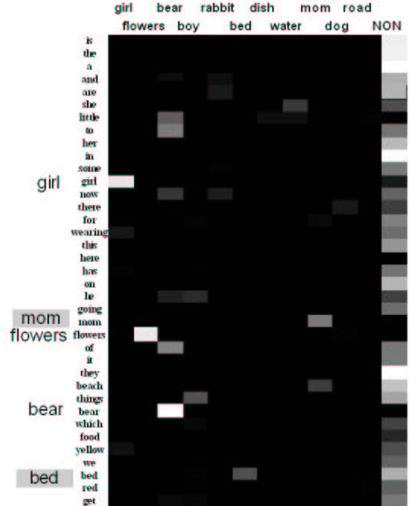
Figure 2: The row is a sorted list of most frequent words and the column is a list of (a subset of) meanings. Each cell is the association probability of a specific word-meaning pair. Dark color means low probability while white means high probability.
